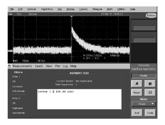
Figure 2-35: Asperity measurement results example
