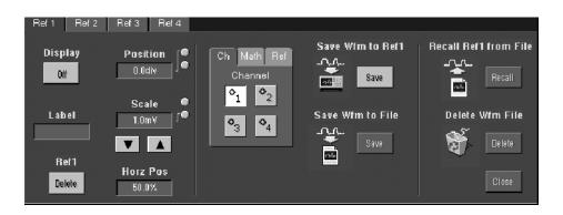
Figure 2-26: Oscilloscope reference waveform setup
