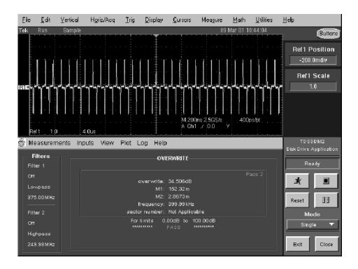
Figure 2-37: Overwrite measurement results, PASS 2 example
