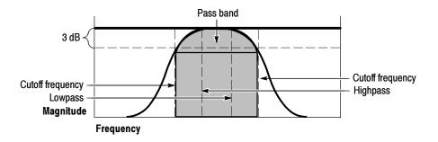
Figure 2-13: Using both Highpass and Lowpass filters
