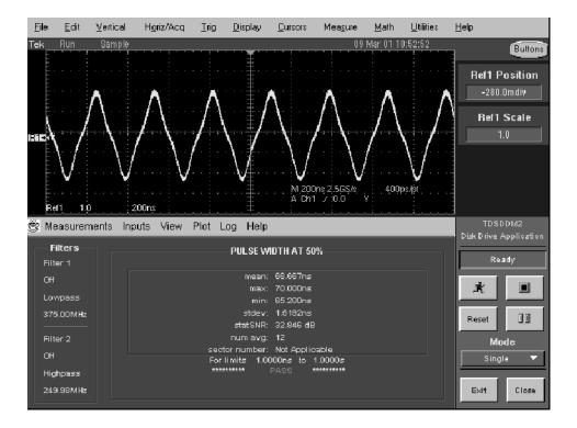
Figure 2-34: PW50 measurement results example
