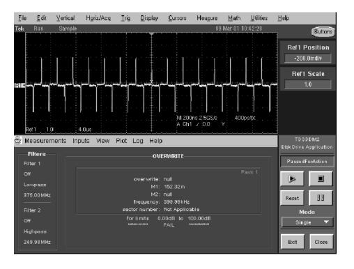
Figure 2-36: Overwrite measurement, PASS 1 example
