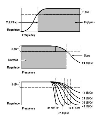
Figure 2-12: Filter characteristics
