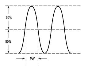
Figure A-3 shows how a pulse width at 50% is defined.
