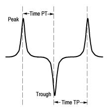
Figure A-6: Time PT and Time TP measurements
