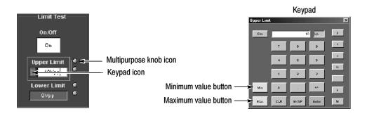
Figure 2-4: How to enter Limit Test option values
