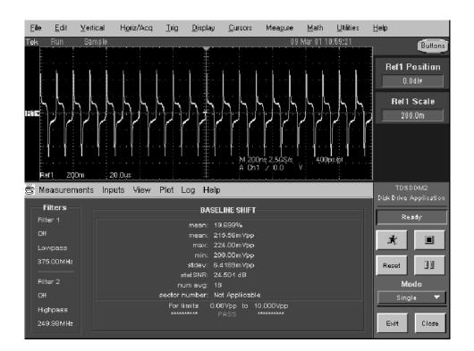
**4.** When the measurement is complete, the statistical results automatically display. Figure 2-38 shows an example of a Baseline Shift measurement results based on the baselineShift.wfm file.
